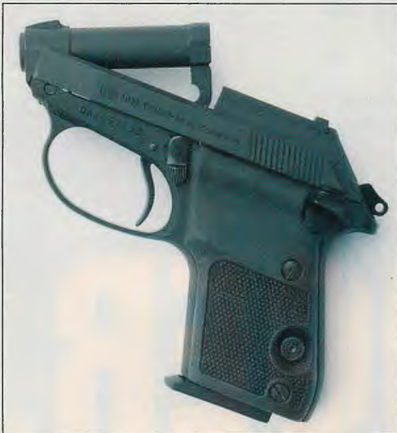
Tip-up barrels are a distinguishing characteristic of all the small Beretta semiautomatic, double-action pocket pistols.
